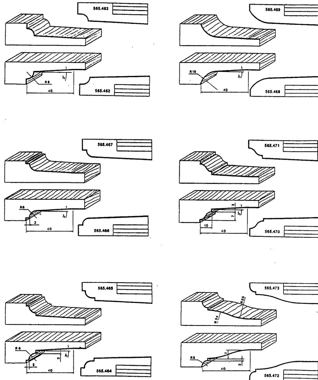
OPTIONS: CES CÔUTEAUX PROFILS ET CONTRE-PROFILS PEUVENT SE MONTER SUR LE DISQUE PRESENT DANS CE COFFRET.
